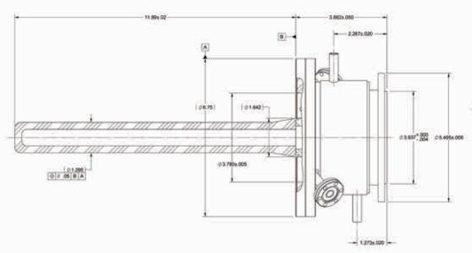
The VWP3143 Power Coupler was designed for ORNL's upgrade to the SNS system, as a higher power variant to the original VWP1133.
